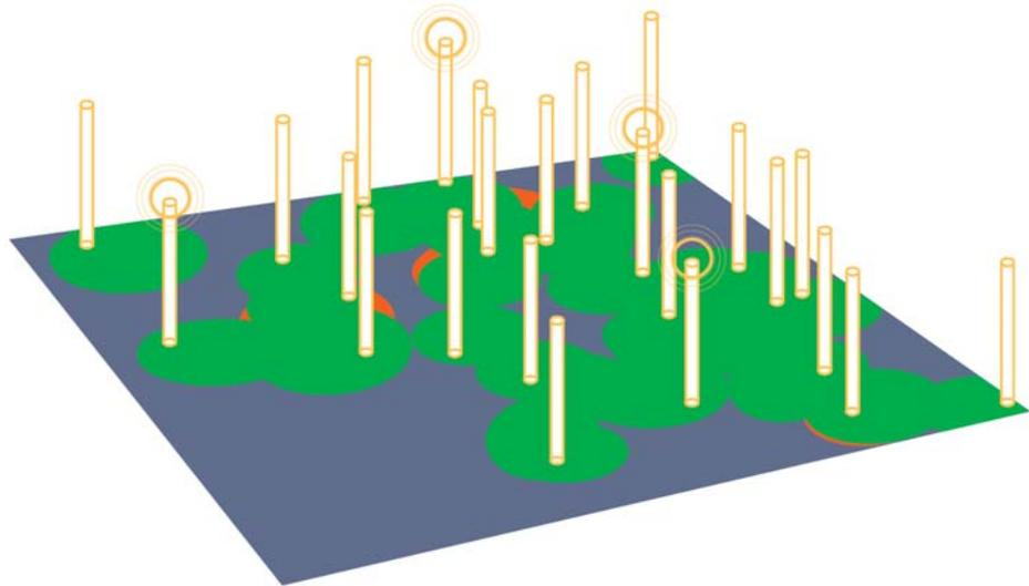
Figure 4b. Canopy coverage in a dense deployment.
