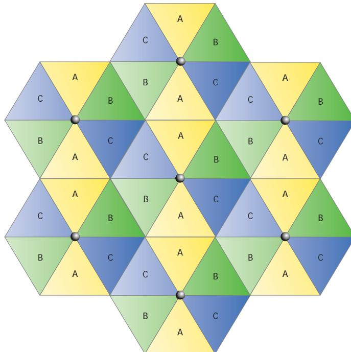
Figure 2. Frequency planning in a cellular deployment.
